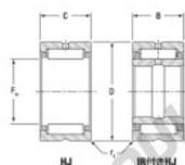
Heavy duty needle roller bearings
