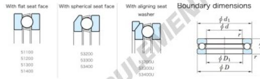
Thrust Ball Bearings - Single Direction
