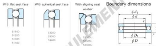
Thrust Ball Bearings - Single Direction
