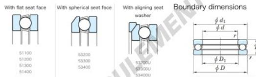
Thrust Ball Bearings - Single Direction
