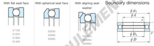
Thrust Ball Bearings - Single Direction
