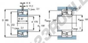
Technical drawing showing dimensions: d=170, D=260, B=67, C=710, C<sub>0</sub>=1060, Vitesse de référence=2200, Vitesse limite=2800. Coefficients de calcul: e=0,23, Y<sub>1</sub>=2,8, Y<sub>2</sub>=4,4, Y<sub>3</sub>=2,8.
